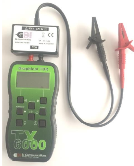
Figure 1 - Connecting Blocking Filter to TDR
